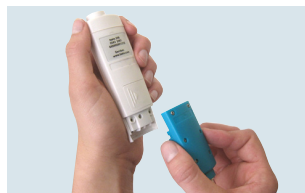
Easy exchange of probes with testo 206-pH1/-pH2/-pH3
